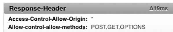
Figure 9: Two additional headers in the HTTP response of Jersey enable client-side cross-origin requests, specified by CORS.
